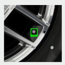
Detection of valve position and presence of valve cap: This feature checks whether the correct valve cap is mounted.
