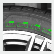
Al-based detection of DOT & DOM on both sides: By using artificial intelligence, DOT/DOM codes on the outer and inner sides of the tire are precisely identified, ensuring complete traceability and compliance.
