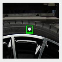
Detection of the position of colored match points on tires and rims: This feature detects the exact positioning of colored match points on the rim and tire, which is crucial for the correct assembly and balancing of the wheels.
