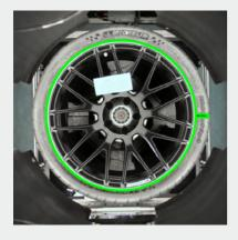
Detection of correct rim design: This test ensures that each wheel is equipped with the specified rim design.
