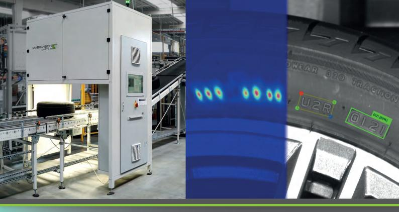
The MV.EYE K2 reading bridge from MABRI.VISION was developed for fast detection and reading of DOT-TIN numbers on tires. Through an innovative imaging concept, the DOT codes are read without handling and without laser at conveyor speeds of up to 1m/s. The application area is in the field.
