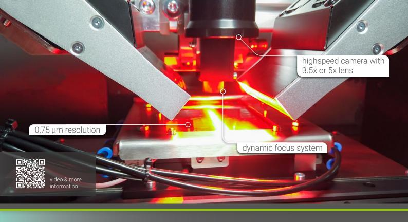
With the MV.EYE MI1 inspection system, MABRI.VISION offers a inline-cabable vision solution for the automated testing of microstructured components. With speeds of up to 40mm/s, the surface structures are displayed in high-contrast thanks to optimized line illumination. Line widths range between 8mm and 25mm.
